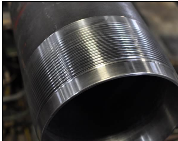
Figure 1, Example of an EVRAZ QB2 Connection That has had the Diameter Machined
